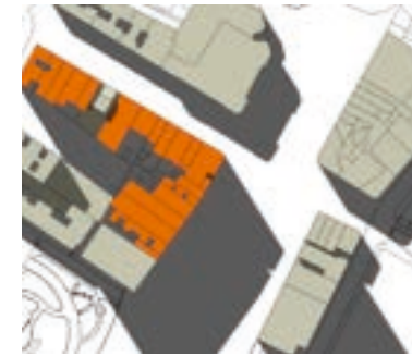
Shadow study 60 m building heights (orange). 2 pm, June 21. Large areas of Anhangabaú are in risk of overshadowing at key times of year.
