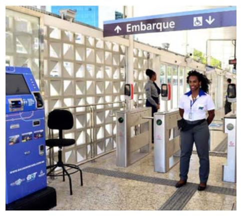
Tactile paving is important to help navigate the visually impared as shown in the Itaigara BRT Station in Salvador, Brazil . **CREDIT:** Jefferson Peixoto
