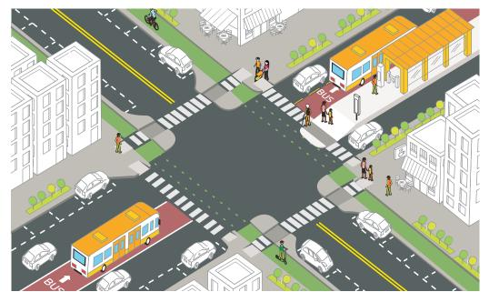
Busway that is split into one-way pairs on separate street and centrally aligned in the roadway
