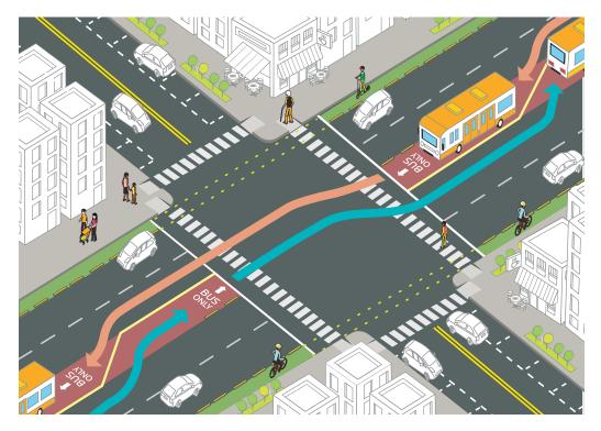
Virtual busway that operates bidirectionally in a single median lane
