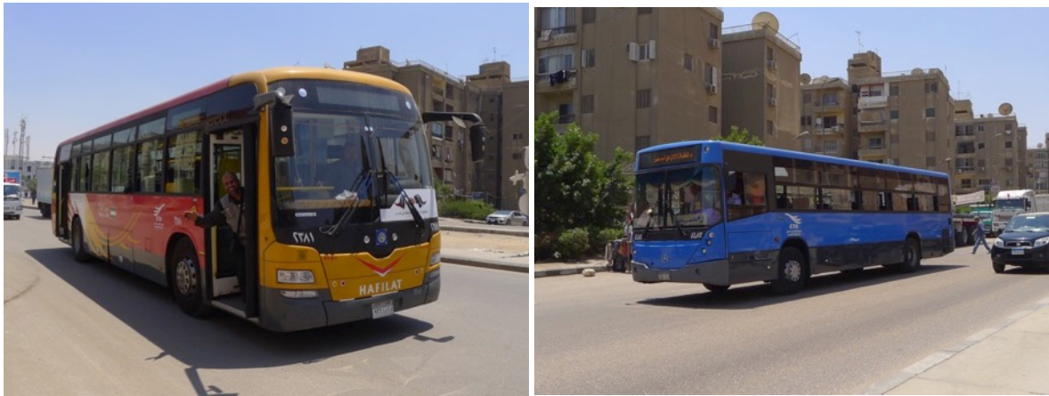
Figure 6: The Cairo Transport Authority (CTA) operates buses across routes in Cairo and Giza. While some vehicles were procured recently, the entire fleet consists of high floor buses with stepped entry.
