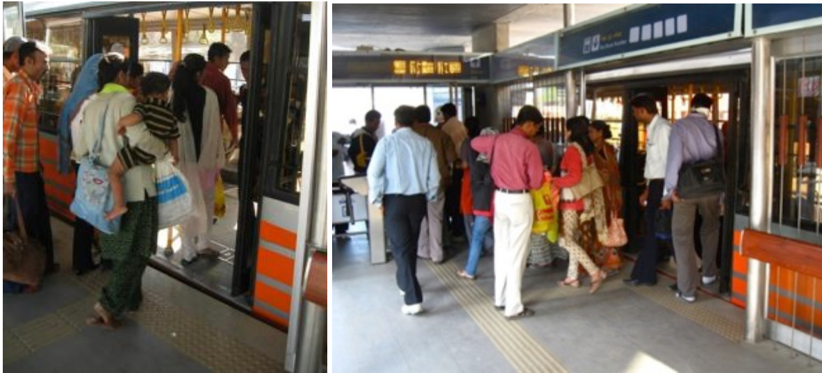
Figure 31: The design of stations and buses must be coordinated to provide level boarding.
